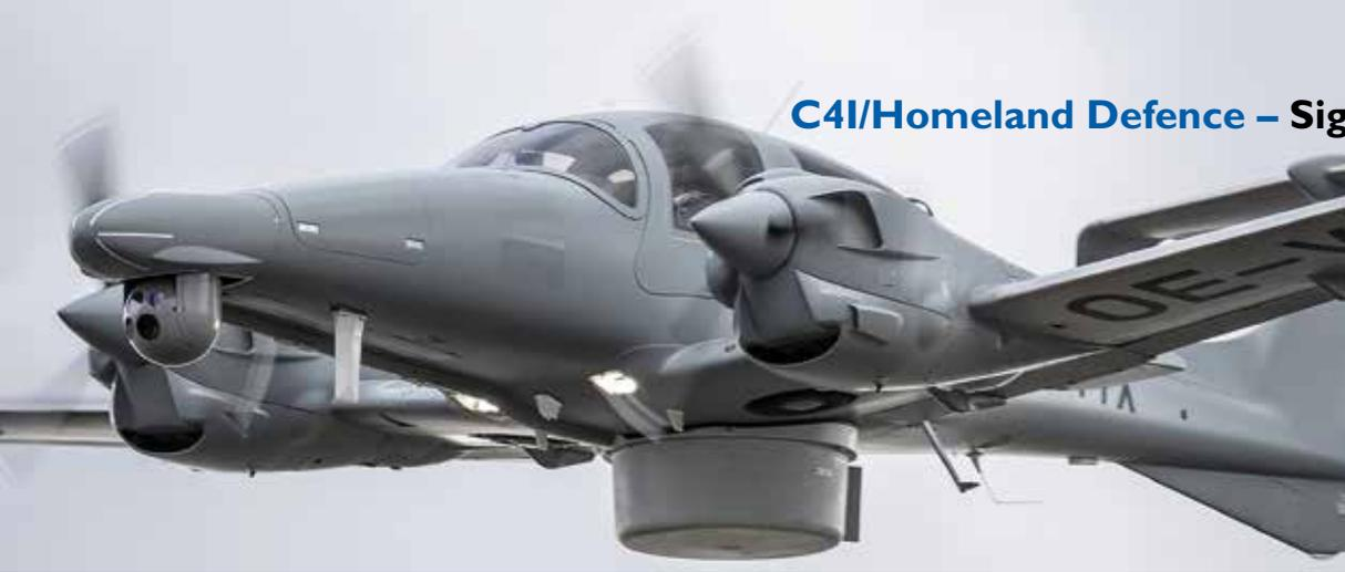
A DA-62 MPP special mission aircraft equipped with a Rohde & Schwarz communications intelligence/counter-ESM system for the detection, analysis and geo-location of signals of interest. The electro-optical/infrared gimbal can be automatically guided to the direction as well as to the source of the signals. (Photos: Diamond Aircraft)
